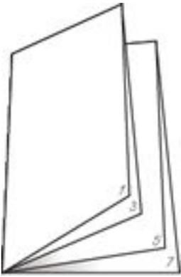
In order to set up your pages correctly, the first step is to create a dummy. A **dummy** is a folded representation of the finished job. To prepare a dummy, fold sheets of paper to obtain the desired number and size of pages, then number them. The odd numbers are always on the right-hand side and the even numbers on the left. Most printers work in 16-page signatures, so the first spread would be pages 16 and 1. It is important to know which page numbers are on which side of the sheet, so if
